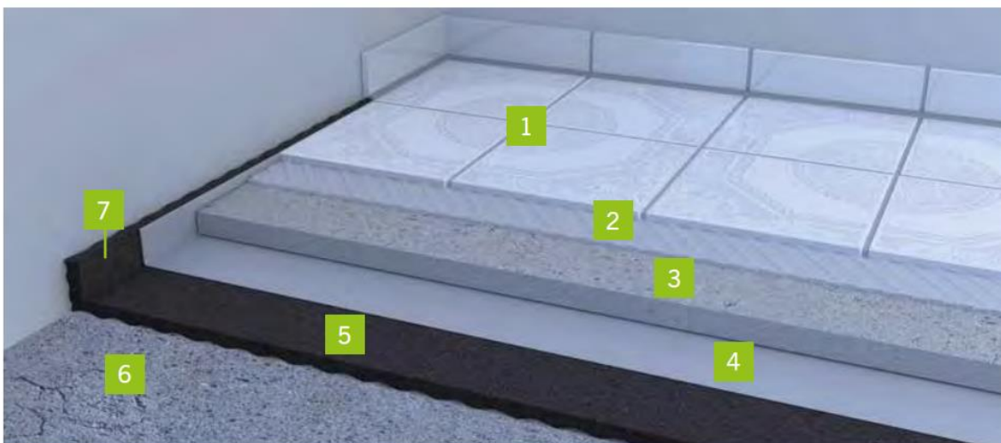
1 tiles or other floor coverings • 2 glue • 3 screed • 4 PE foil • 5 Regupol® or Regufoam® screed insulation • 6 raw ceiling • 7 perimeter insulation strips made of Regupol® , Regufoam® or another material
